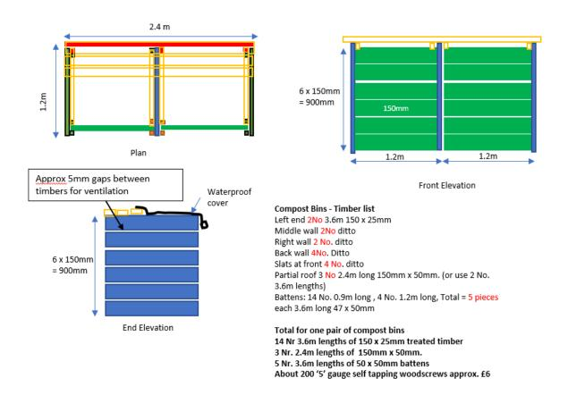
All timber FSC certified, pressure treated for use in contact with ground.
